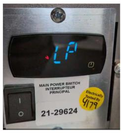
If you are experiencing issues with your equipment not maintaining temperature, check the magnetic filter and condenser coil surfaces and take the following steps prior to calling for service.
